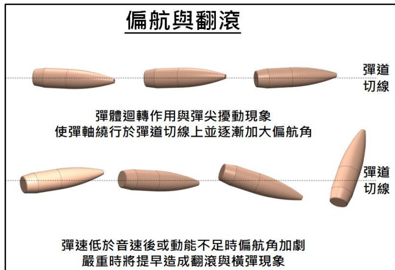
Fig. 8 Schematic diagram of the "yaw and roll" phenomenon of the warhead flight (Adapted by the authors).
