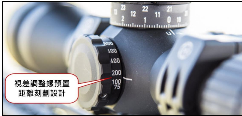
Figure 17 Parallax Adjustment Screw and Distance Scoring Source: Photographed by the author (September 28, 2021)
