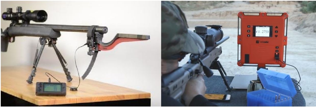
Figure 13 Muzzle Electromagnetic (MagnetoSpeed) and LabRadar Tachometers Source: http://www.3gsports.de <MagnetoSpeed V3 Chronograph> and http://www.ocabj.net <LabRadar Chronograph Review> (Retrieved 2021 (September 16, 2011)
